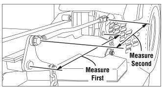
Figure 39. Check Lift Rod Timing
